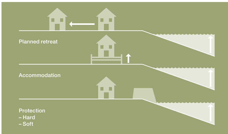
Figure 5.1 An illustration of the possible adaptation responses to sea-level rise
